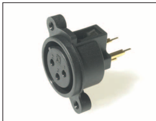
XNACF4V - 3 Pin vertical PCB mounting Female XLR with latch. Gold plated PbRz contacts standard.
