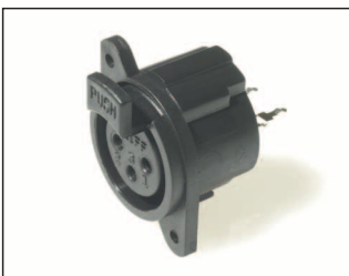
XNACF3V - 3 Pin vertical PCB mounting Female XLR with latch. Nickel Silver or Gold plated PbRz contacts available.
