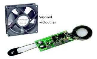
This automatic temperature controller is designed for miniature DC fans (12 V) used in almost all PC computers. The temperature sensor controls the speed of the fan according to the temperature.
