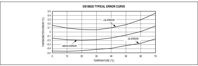
Figure 1. Typical Performance Curve
