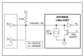
Figure 12. Hardware Configuration
