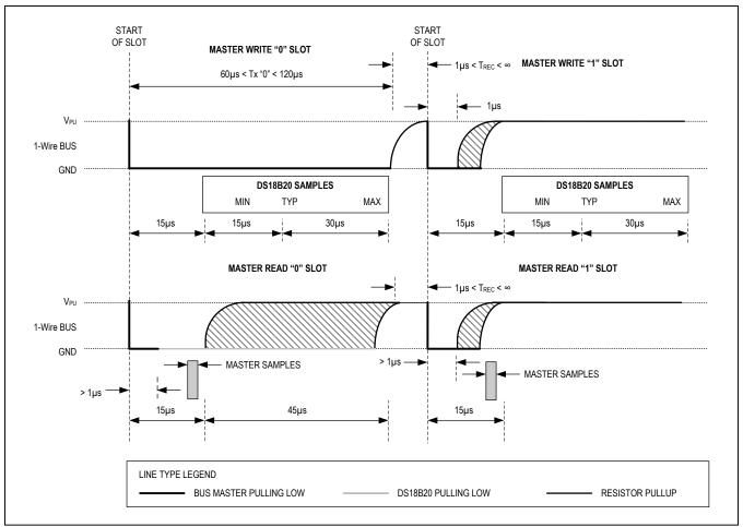
Figure 16. Read/Write Time Slot Timing Diagram
