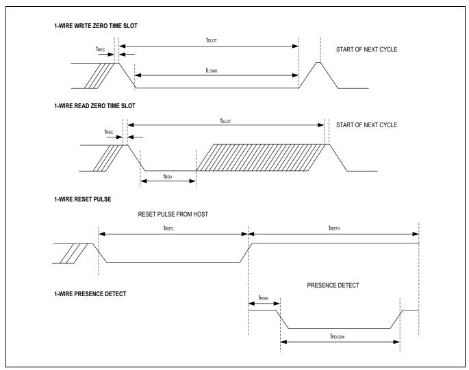
Figure 2. Timing Diagrams
