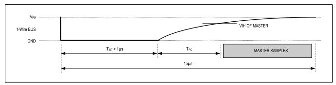
Figure 17. Detailed Master Read 1 Timing
