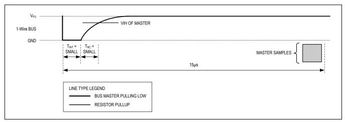
Figure 18. Recommended Master Read 1 Timing
