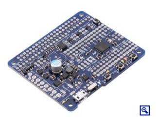
Like other **A-Star programmable controllers** [https://www.pololu.com/category/149/a-star-programmable-controllers] (abbreviated A\*), the robot controller features a USB interface and ships with a preloaded Arduino-compatible bootloader. We provide a software add-on that enables it to be easily programmed from the Arduino environment, as well as an Arduino library to help interface with its on-board hardware.
