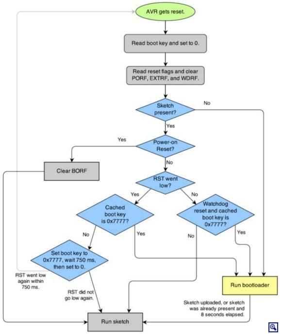
The startup logic for the A-Star 32U4 bootloader.
