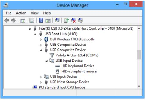
The Windows 8 Device Manager in "Devices by connection" mode, showing that the A-Star is a composite device.
