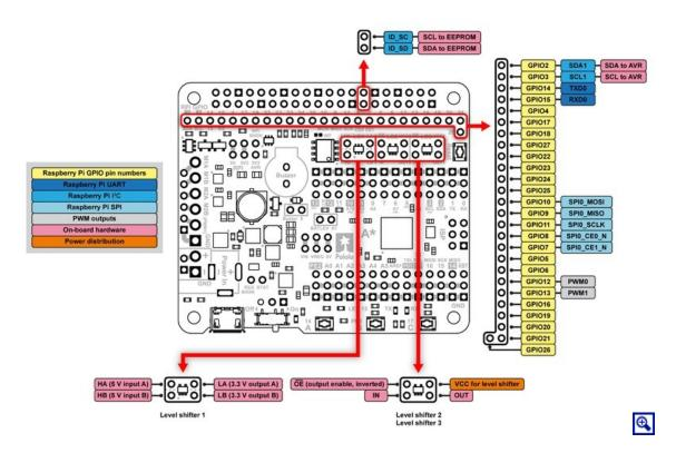
Printed on the A\* circuit board are indicators that you can use to quickly identify each AVR I/O pin's capabilities: an analog pin number (prefixed by the letter A) means the pin can be used as an analog input, and a square wave symbol next to the hole pair means the pin can be used as a PWM output. Pin numbers printed as inverted text surrounded by a white box indicate that the pin is used by on-board hardware (see **Section 3.7** for more information about pin assignments).
