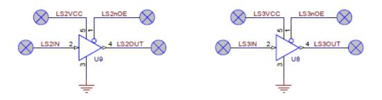
For example, if you pull  $\overline{OE}$  low, connect a 3.3 V signal to IN, and connect 5V to VCC, the signal will be shifted to 5 V logic level on OUT.
