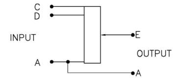
Connection 230V on A - C delivers max. 230V output A – E. Connection 230V on A - D delivers max. 260V output A – E.
